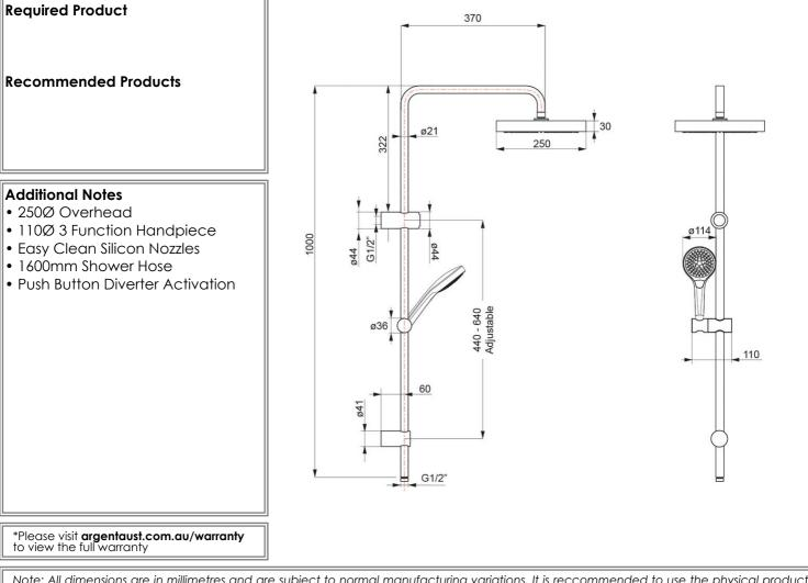
Note: All dimensions are in millimetres and are subject to normal manufacturing variations. It is reccommended to use the physical product measurements for cut-outs and rough-ins as the technical details shown may differ from the actual product. Use acetic cured silicone sealant. Do not use epoxy type adhesives. Clean with damp cloth. Do not use abrasive cleaners, liquids or pastes.
